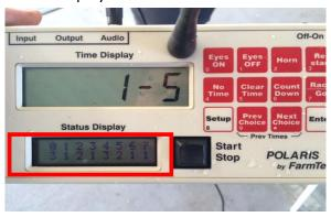
In the status display the top row are the channels being used by the system, (eg pass pole, start pole, judges remote etc) and the bottom row shows the level of interference on each channel.
