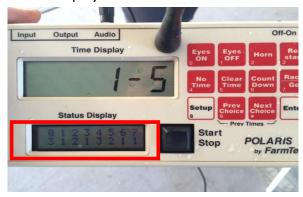
In the status display the top row are the channels being used by the system, (eg pass pole, start pole, judges remote etc) and the bottom row shows the level of interference on each channel.
